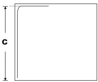
C = measurement from the floor to the roll up door track at the rear before the curve to the vertical door track
